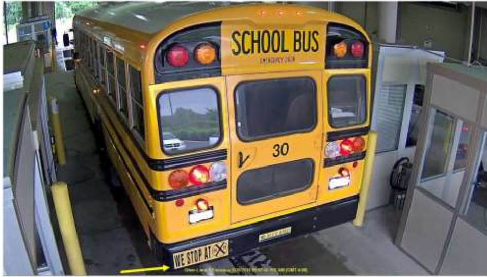
Location of "We Stop at R/R Crossings" on buses manufactured after Jan. 1, 2012
